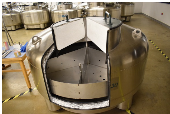
Photo 5: Dissected 1500lt liquid nitrogen dewar showing the turn table on which sample racks are housed and thick isolation to maintain temperatures at -196^{\circ}\text{C} .
